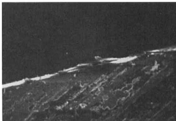
a) Typical porous surface texture and morphology for the formed coatings at 250x.
